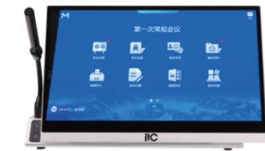
TS-8515M3 Desktop Dual Screen Paperless Monitor with Microphone
